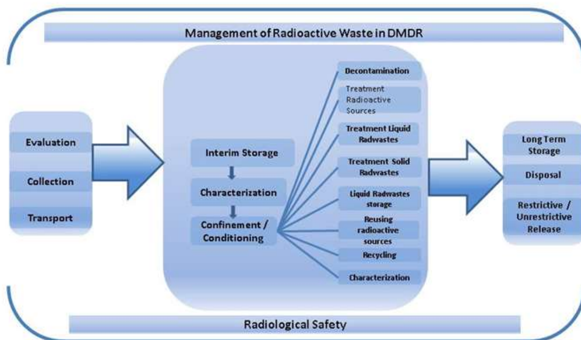
Figure B8: IFIN-HH Radioactive waste management scheme
