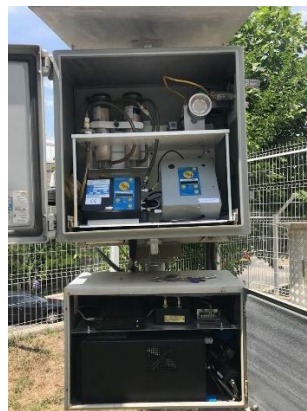
Figure 2.4 - F&J fixed low flow (10 l/min) sampling station, model LV118ECNV CAS
